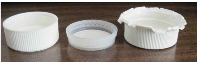
Child proof top, inner assembly, remains of child proof top
